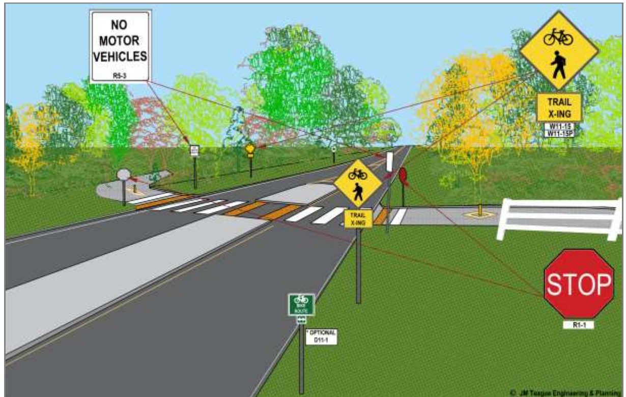
Exhibit 8-5: Typical Crossing Treatment for Multi-Use Trail at a Two-lane Road
